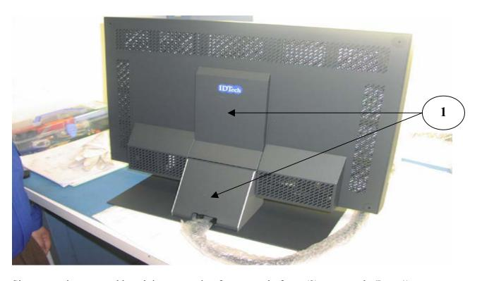
Situate monitor on workbench in preparation for removal of two (2) rear panels (Item 1)
