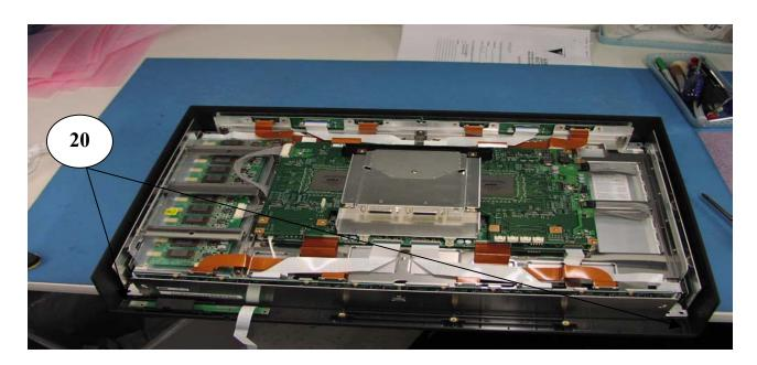
Carefully lower panel into bezel (Item 20), ensuring the panel drops into the bezel guide pins.
