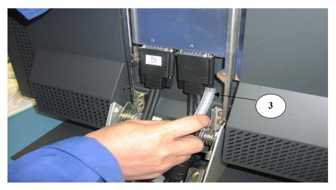
After second panel is removed, use a tube (Item 3) to loosen the four (4) connector mounting screws.
