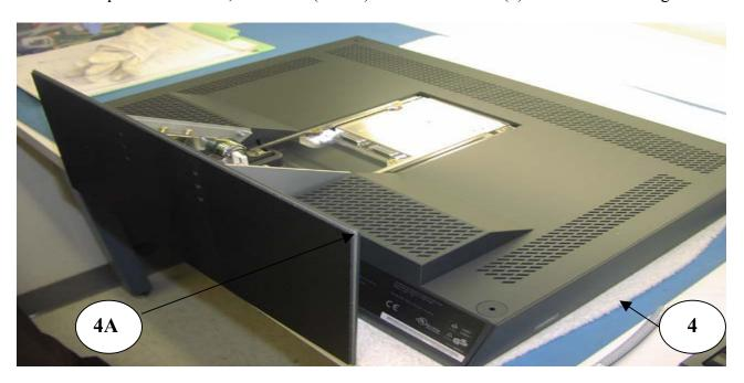
Once both cables are removed from the monitor, lay monitor on bench with screen surface down (protected by foam- Item 4) in preparation for removal of base (Item 4A).
